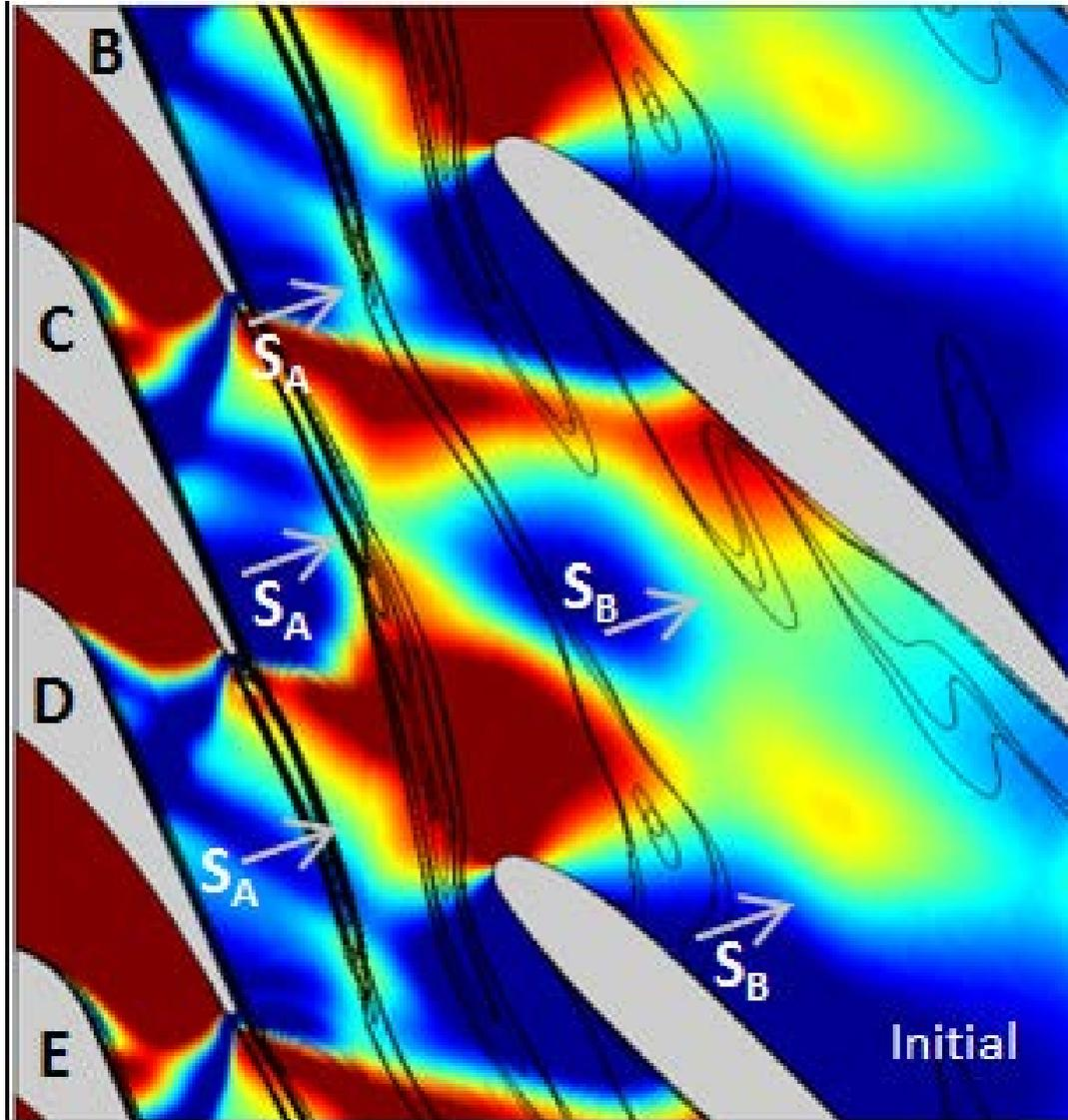
Reflected shocks are labeled with subscripts indicating originating blade, e.g.
