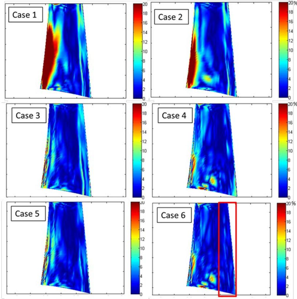
Differences of the Normalized DFT Magnitudes at 46E of the Full-Wheel Simulation and Each Sector as a Percentage of the Maximum Unsteadiness of the Full-Wheel Simulation
