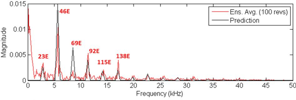
Experimental and Predicted DFT of PRZA14 (Blade SS, 15% Span, 87.7% Axial Chord)
