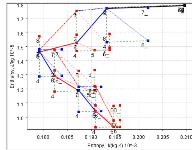
Enthalpy-Entropy Diagram of uncooled & cooled turbine
