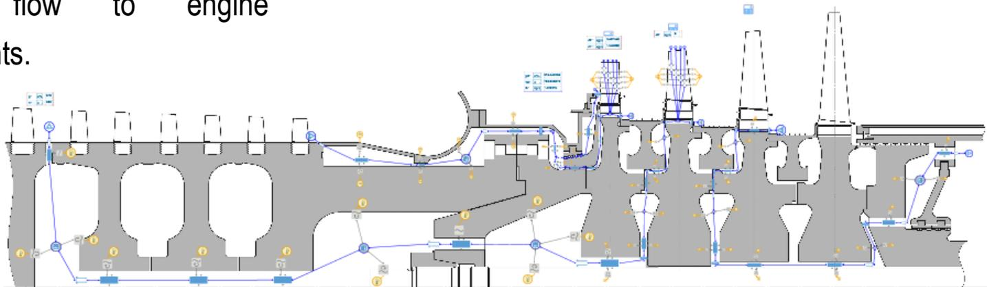
Scheme of secondary flows in a gas turbine engine
