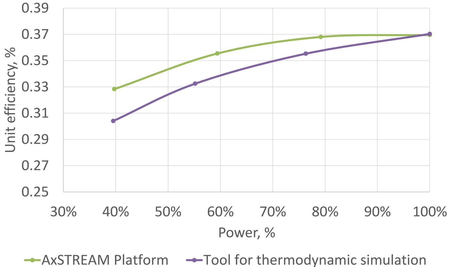
Figure -The dependency of unit efficiency from power level
