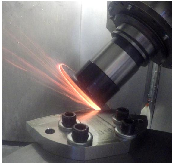
Figure 1: Example for new roughing strategies on Blisk segment demonstrator: ceramic disk cutter for slot opening
