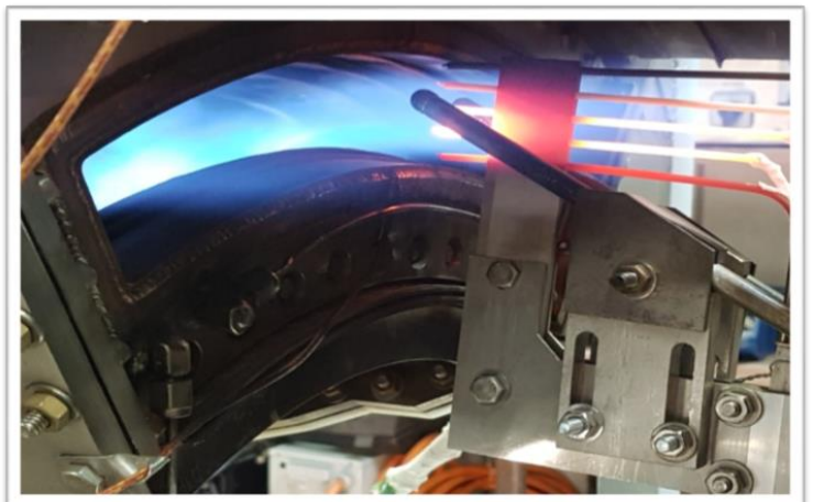
Combustor operating with methane fuel
