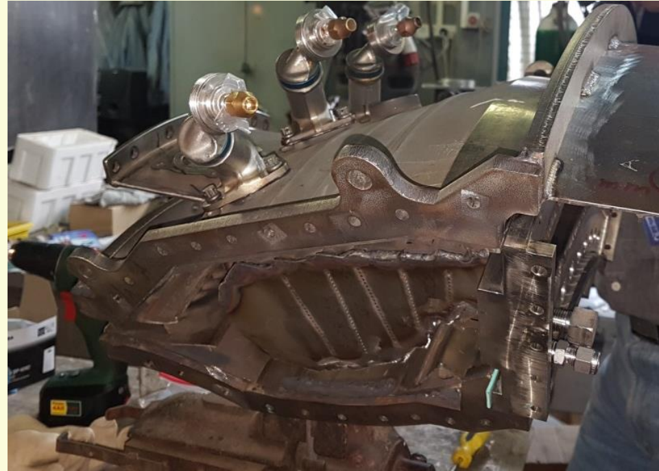
The liner and outer case sector with 3 fuel nozzles installed. (without outer side walls)
