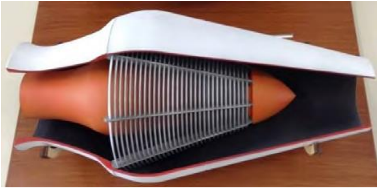
Fig 4a: CORN (COncal Recuperative Nozzle)
